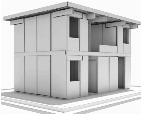
SECU – emerging city unit out of prefab straw boards (realised in April 2012)
